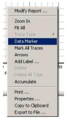
Select a point as close as possible to zero along the imaginary line. You will not be able to choose exactly zero due to the resolution chosen (1000 points) in the solution setup. Left-click to mark the point as shown below:
