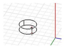
Follow the format below for structure size. Give the name dip1 to this object. Assign the material PEC and click  $\mathbb{OK}$ . PEC (Perfect Electric Conductor) will create ideal conditions for the element.
