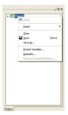
To begin working with geometries, you must insert an HFSS design. Right-Click the project file and select Insert -> Insert HFSS Design from the menu.
