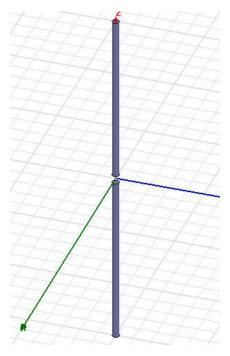
Ideally, the structure is one solid geometry. A slot has been created at the origin in this example. This will allow later placement of a source for excitation.
