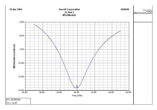
The point of resonance was marked at -14.57dB. In order to compute accurate antenna parameters, the input must be matched. From the project explorer, right-click *source* and select Properties. Adjust the port impedance as shown:
