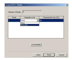
Using the mouse, position the cursor to the bottom-center of the port. Ansoft's snap feature should place the pointer when the user approaches the center of any object. Left-click to define the origin of the E-field vector. Move the cursor to the top-center of the port. Left-click to terminate the E-field vector. Click finish to complete the port excitation.
