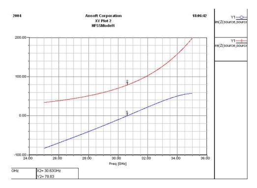
The input resistance of the antenna is 78.83 ohms according to the graph. Performing calculations from a text, the user should compute a resistance between 65 and 75 ohms. The port was previously defined with an impedance of 50 ohms. This will produce sub-optimal results due to mismatched impedance. This will be corrected shortly.
