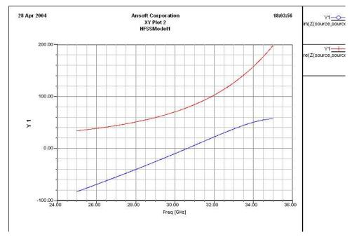
The input resistance can be directly determined from the graph. We will mark the point at which imaginary component crosses zero. This mark will allow the user to determine input impedance at the point of resonance. Right-Click the graph and select  $\mathbb{Z}_0$   $\mathbb{I}_n$ .
