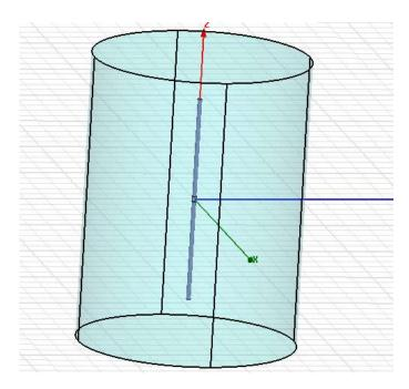
With the geometry complete, the actual radiation boundary may now be assigned. From the 3D toolbar select face from the drop down window as shown below.
