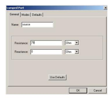
We will now re-analyze the structure with a properly matched port. In order to preserve memory and calculation time, right-click Analysis -> Revert to Initial Mesh in the project explorer.
