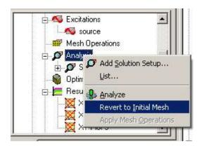
Re-analyze the structure. When complete create another plot of  $S_{11}$  vs. frequency as shown below:
