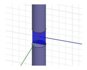
With the source geometry in place, the user must provide an excitation. A lumped port will be used for the dipole model. This excitation is commonly used when the far field region is of primary interest. In the project explorer, right-click Excitation -> Assign -> Lumped Port.
