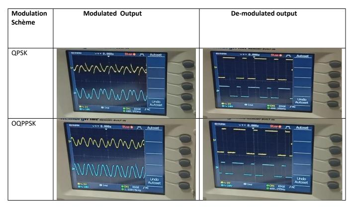
**Results** - By using the **2808 kit**, we observe input data at TP2, 2-bit encoded input data at TP4, sinusoidal carrier signal at TP6 & TP7, modulated output at TP9, and de-modulated output at TP18. In the same way, we can observe output for OQPSK at different terminal points. Accordingly, modulated and demodulated output graphs are plotted in observation table.
