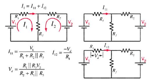
$R_i || R_i$  means the parallel resistance of  $R_i$  and  $R_j$  .
