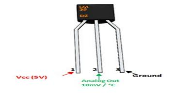
**Observation :** We have used LM-35 and op-amp 741 IC to compare the out put voltage of LM-35 with the reference voltage. We have set up the circuit so as to trigger the LED to glow when the temperature is greater than  $28^{\circ}$ C.
