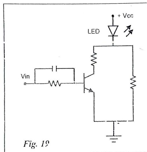
Fig. 19 shows a simple drive circuit for binary digital transmission consisting a common emitter - saturating switch.
