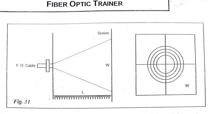
5. Record the distances of screen fro the fiber end L and note the diameter W of the spot.
