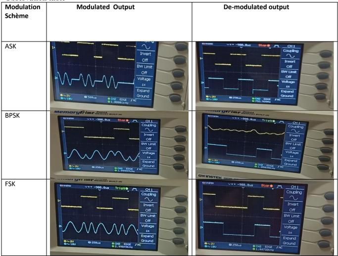
**Results** - By using the **2807 kit**, we observe input data at TP2, 1-bit encoded input data at TP3, modulated output at TP5, and integrator output at TP7. Similarly, we observe output at different terminal point for PSK and FSK. Accordingly, modulated and integrator output graphs are plotted in observation table.
