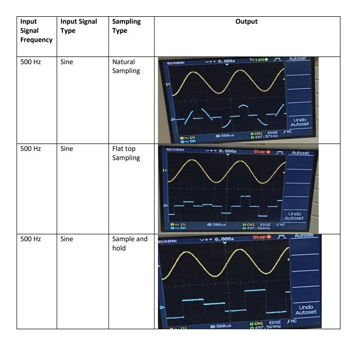
**Results -** In this exercise, we observe that the PAM signals consist of samples of the message signal. Moreover, we have observed the differences between natural, flat-top, and sample & hold sampling using different sampling rates and pulse-widths.
